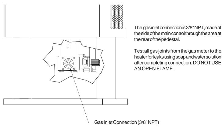
FIGURE 6. Rear View of 9945 Vent-Free Gas Heater
